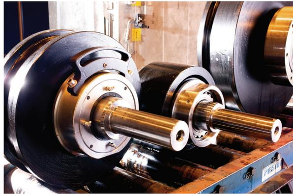
At the steel mill, bridge wheel flanges started breaking off and falling 40 feet to the work area below. This caused a major safety concern for the mill.
